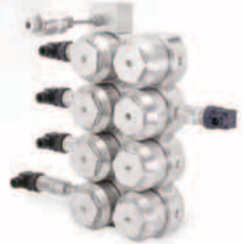
High pressure valve manifold used to calibrate transducers
